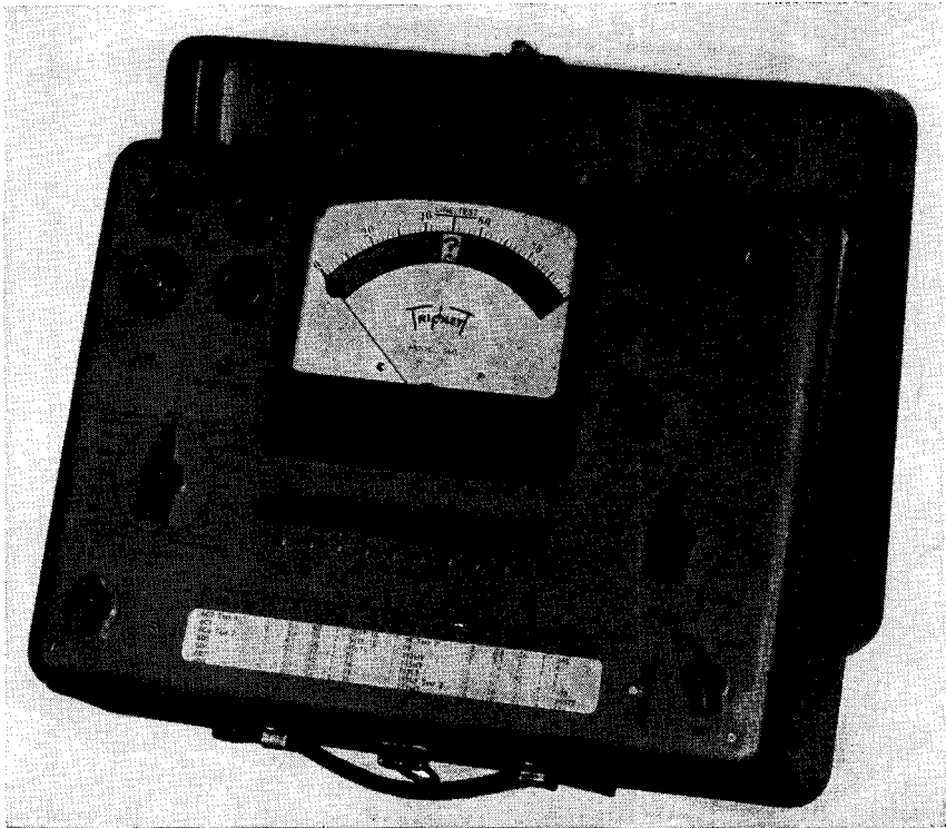
Fig. 1. Example of good tube tester using lever switching. In this Triplet model 3413 tester, the roll chart is visible through a window at the bottom of the tester panel and is moved by spinning the knurled wheel projecting up through the panel at right of chart. (Triplet photo)
