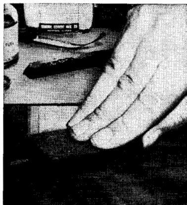
Fig. 4. Rubbing hardened stick shellac in scratch with felt pad moistened with shellac rubbing fluid, to make the repair level with the surrounding finish. (General Cement photo)
