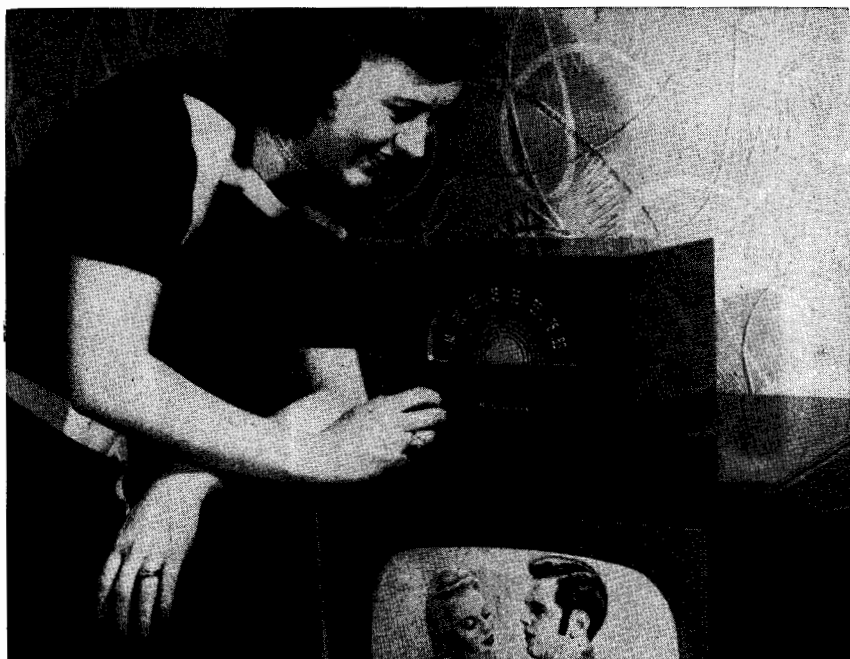
Fig. 9. Converter unit being used with vhf television receiver to bring in uhf stations. Dial is marked in uhf channel numbers from 14 to 83. (RCA Victor photo)
