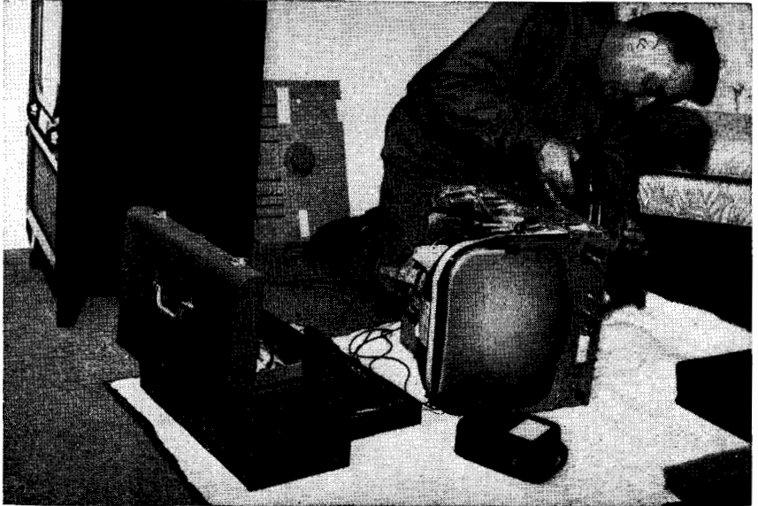
Fig. 1. Installing new carbon resistor in television receiver in customer's home. Note use of blanket-type pad under receiver and toolbox. (Electrical Merchandising photo)
