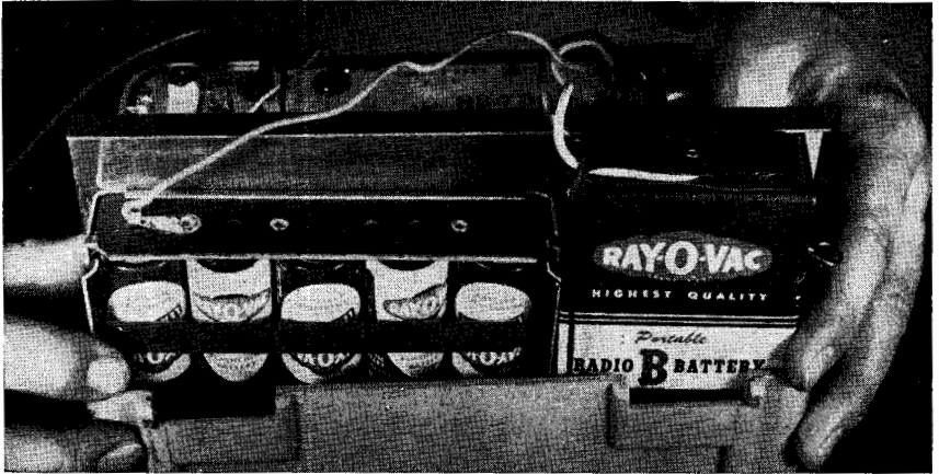
Fig. 8. Inserting tray of new batteries in cabinet of three-way portable, after tying the 67½-volt B battery to the tray with a piece of wire. The five flashlight cells are installed with caps alternately up and down to provide the required series connection for 7½ volts. Always note battery positions carefully before removing them. (Ray-O-Vac photo)
