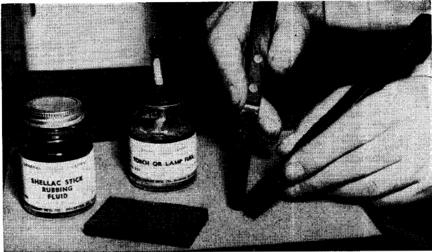
Fig. 2. Applying stick shellac to blade of spatula after heating the blade in the flame of an alcohol lamp, for use in filling deep gouges in a cabinet. (General Cement photo)
