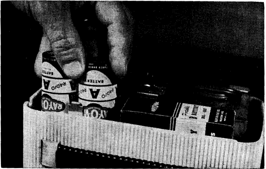
Fig. 6. Three-way personal portable radio, showing how flashlight-cell A batteries are installed. Connections are made automatically by spring clips when cells are pushed in and cover of set is replaced. The B battery, at right of cells, has snap connections. (Ray-O-Vac photo)
