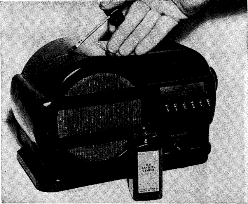
Fig. 5. Applying special plastic cement to a crack in a plastic radio cabinet. To be effective, the cement must be worked into the crack. (General Cement photo)
