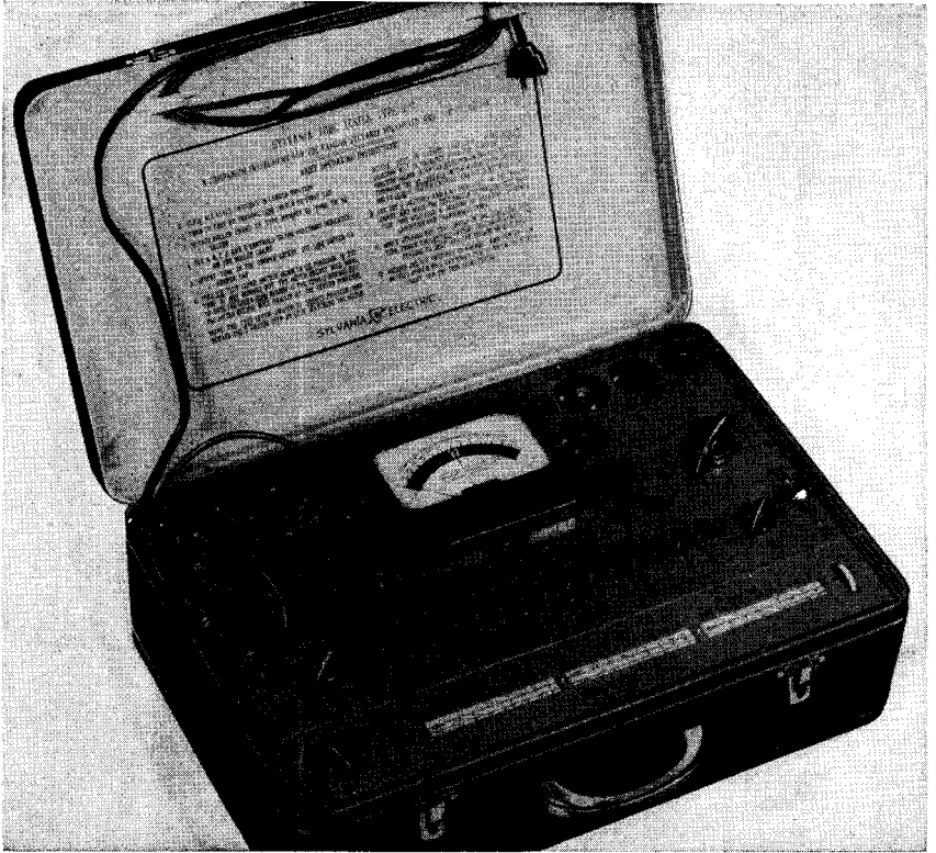
Fig. 4. Example of good portable tube tester having operating instructions printed directly on inside of cover where they cannot get lost. This is a Sylvania model 220 tester, having lever switching and a three-section roll chart. (Sylvania photo)
