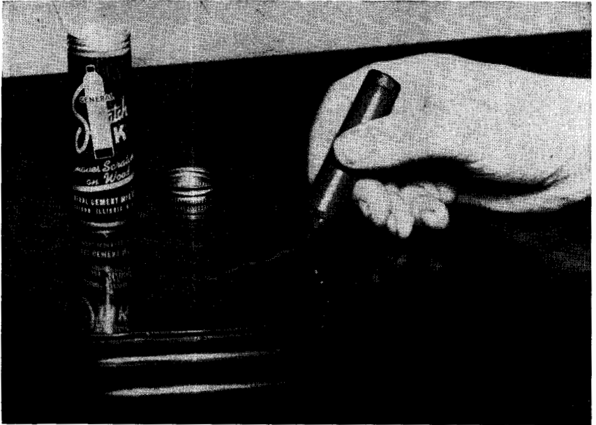
Fig. 1. Using a scratch stick to touch up scratches on a wood cabinet. (General Cement photo)
