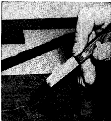
Fig. 3. Spreading molten shellac into deep scratch with spatula. (General Cement photo)
