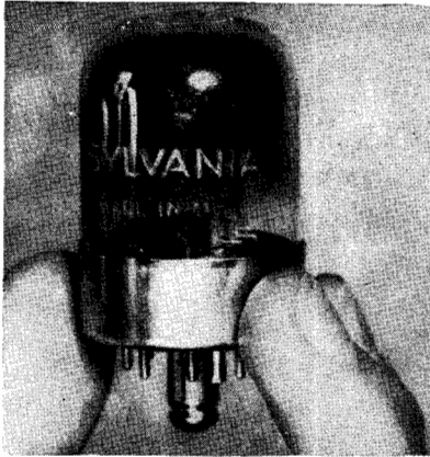
Fig. 5. Example of a 6X4 tube, showing glass envelope, metal base, metal aligning key, and solid wire pins that go right through the glass envelope. (Sylvania photo)
